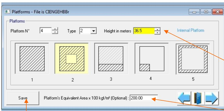
For platforms, the choice is simple with the help of schematic drawings. Type 5 is a platform outside the tower whereas the others are inside the tower.
